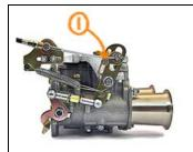
1. **SET the throttle pedal travel** – Unscrew throttle plate idle screw until it is clear of the new carburettor lever so that the throttle plates can completely close. Slacken bolt on cable clamp carrier with the Allen key supplied. **Slide** the whole cable clamp assembly along the slots until throttle fully open and throttle fully closed positions are achieved. Tighten bolt, then locknut.
