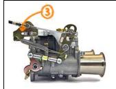
3. **SET the spring tension –** slacken the nuts on the spring/swivelling cable adjuster carrier plate. Slide plate along slot until a good balance between a positive idle shut-off and pedal feel is obtained. Tighten nuts.
