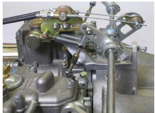
**“Sliding set-up”- simplicity to set (twin cable system only) Full instructions supplied.**
