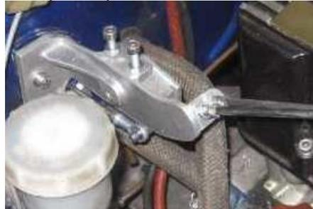
An important feature is the adjustable **fully closed** and **fully open** throttle stops. This enables selection of pedal travel and also pedal position in relation to the brake pedal. This system is ideal for competition use damage to the linkage.
