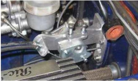
Three bolts fix to bulkhead – template and drill supplied
