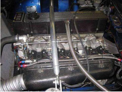
With the accelerator pedal and linkage quadrant in the **fully closed** position, run the cables from the bulkhead bracket to the linkage assembly through the cable support bar, as illustrated. At this stage do not clamp up the inner cables.
