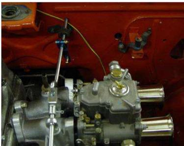
There is much debate about whether a rod or cable linkage is superior. Both are supplied - so you can decide. Our freely rotating, aircraft quality, rose jointed hex bar links, sliding pull-off spring and pedal stop, all contribute to a superior rod linkage over others on the market.
